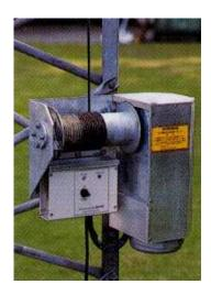
This ED-150 is the winch of electric motor type, that can drive to ascend and descend the elevator truck easily and speedy.
