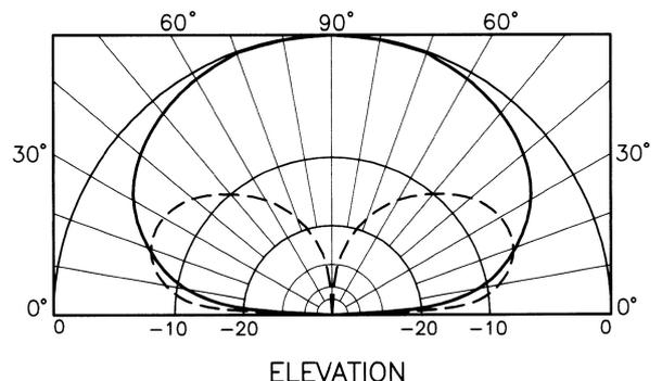
Figure A. CD160L, Radiation Pattern of Reduced Dipole
