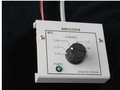
● The CD78-series is a relay controlled, fractional reduced-scaled type of rotary dipole antenna for the operation of 3.5/3.8MHz bands. By applying with a newly developed a High Q loading coil and power durability and capacity hat, it makes it possible to offer high radiation efficiency. Each model comes with 5-CH tune coupler BS81C standard. A 13.8V DC power supply for band switching and control cable of 6-conduct is required (customer furnished).
